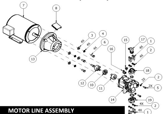
PART # ML-1 (3HP; 3PH; 50/60HZ) PART # ML-4 (5HP; 3PH; 50/60HZ)
