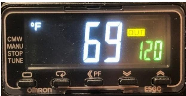
**NOTE!** The Temperature Controller displays the actual material temperature and the set point. The YELLOW box with the word OUT indicates that the heaters are being powered.
