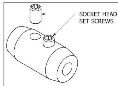
**NOTE!** A good practice is to add some dielectric grease (Permatex 67VR or equivalent) to the outside of the Terminal, where the electrical connection is made, prior to insertion.
