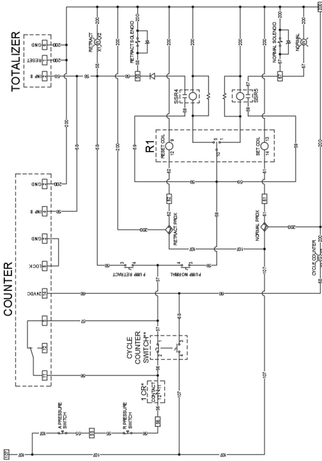
\*See Pressure Balance Control Circuit (Pg. 23) for complete 1 CR wire connections
