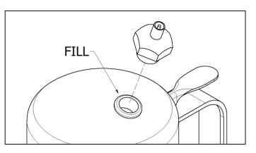
**WARNING!** Do not exceed 200 PSI (13.8 bar) of air pressure. Always check the pressure of the air supply before pressurizing.
